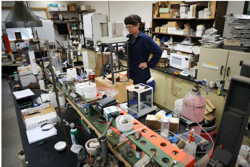
In the Soil Lab, Forest Service biological science technician Courtney Johnson measures the bulk density of sticks collected at sites across the Northern Rockies.
