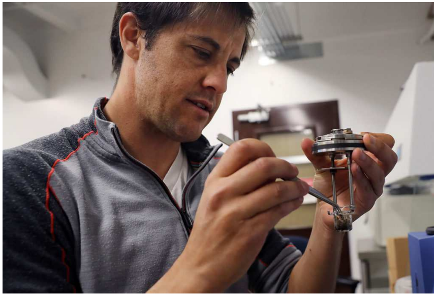
Forest Service Biological Science Technician Elliott Conrad measures the heat content in a sample of live jack pine needles from Wisconsin.
